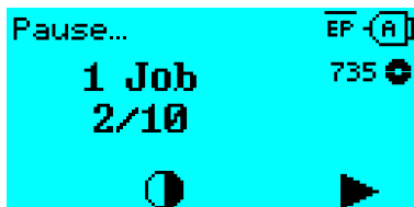
Fig. 55: Stopped print job. Press key 4 to continue printing.
