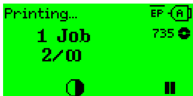
Fig. 54: Print job with endless print amount.
