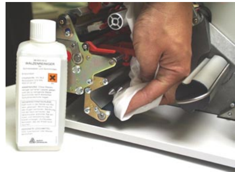
Fig. 6 Left side: pulling out the pull-out module; right side: cleaning the dispenser-feed-roller using roller cleaner.
