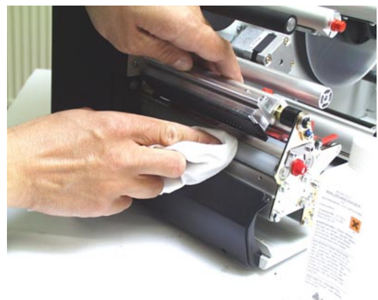
Fig. 4 Rotate the printhead upwards before cleaning it.
