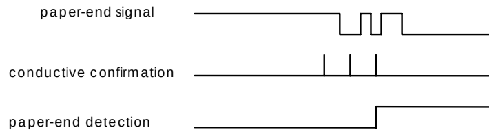
Figure 2-12 Paper-end detector operation
