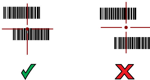
Figure 15 RS5100 Pick List Mode with Multiple Barcodes in Aiming Pattern
