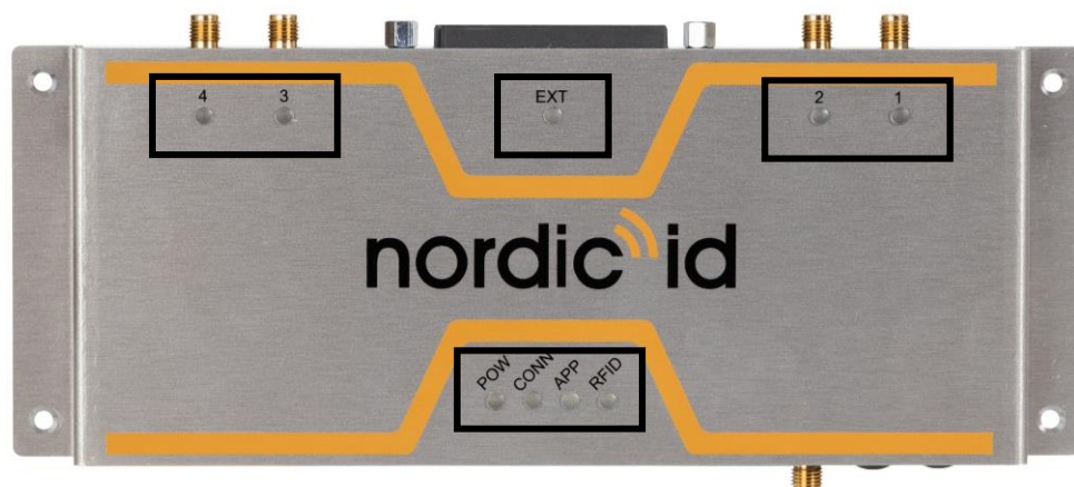
Picture 12 Location of LEDs
